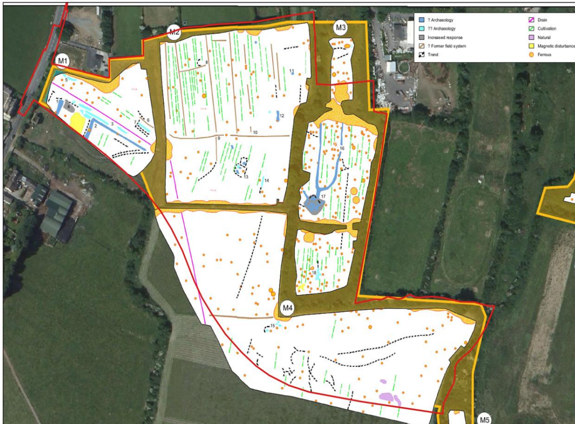
Figure 13.3 - Results of geophysical survey carried out within the proposed development area in 2018
